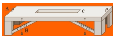
Figure D.15: Chorabates: A - sights, B - weighted strings and notches and C - central channel. ( http://roma.andreapollett.com )
