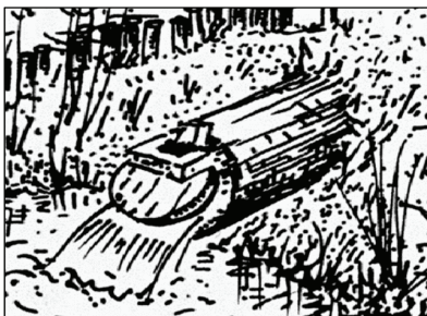
Example of an one way valve (Roman drain pipe in Vlaardingen, Netherlands) (Van de Ven 2003, pag. 12).
