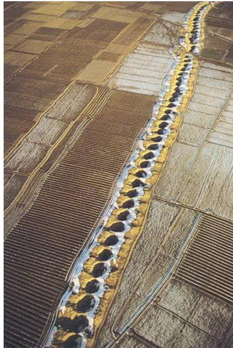
**Fig. 3 (right):** What looks like a line of craters is in fact an aerial view on the tops of the access shafts of a subterranean qanat. (source: [www.muslimheritage.com](http://www.muslimheritage.com)).
