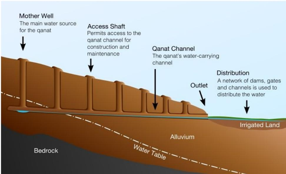
**Fig. 1:** The basic scheme of a qanat (the horizontal channel) with at left the aquifer and the mother well and at right the outlet where the water distribution takes place. Note the many vertical access shafts (source: Wikipedia).
