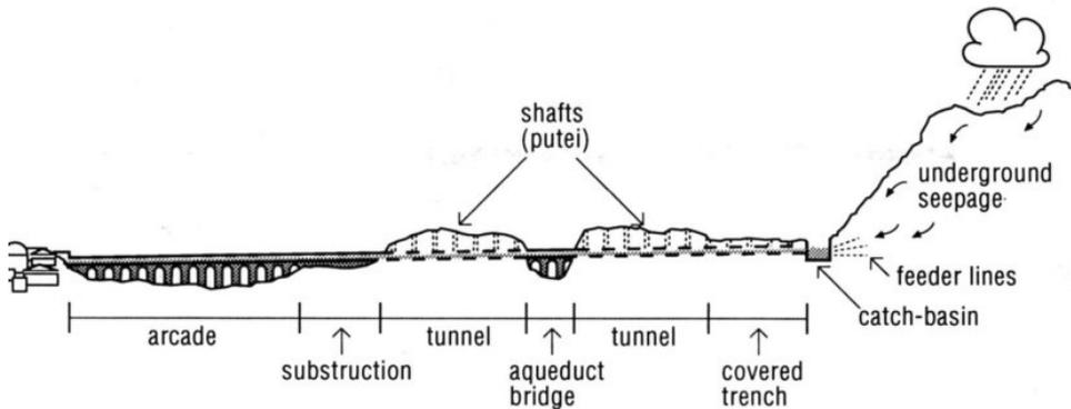
**Fig. 9: The basic scheme of an aqueduct with at right the source (a river tap, spring or dam) and at left a basin where the water is distributed among the users. Do realize that 80% of the course of an aqueduct is subterranean and laid in a covered trench. Note the works of art: arcades, tunnels and bridges. (Drawing from: P.J. Aicher (1995): Guide to the aqueducts of ancient Rome).**
